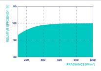
Typical module performance under low irradiance conditions in comparison to STC conditions ( $25 \,^\circ C$ ,  $1000 \, W/m^2$ ).
